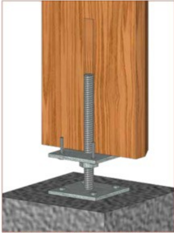
Figure 02-01a. Detail of the vertical cross-section through a simple screw jack installed at the bottom of log post.
